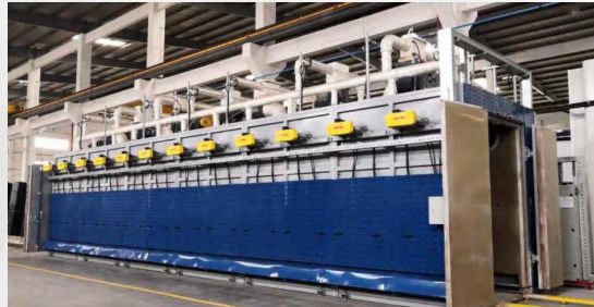
Heat Soaking Test
